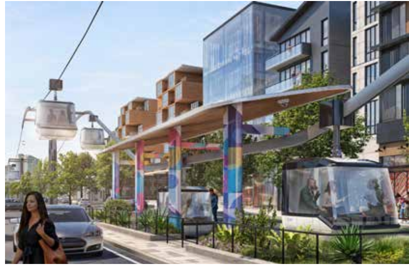
Rendering of autonomous gondolas bypassing intermediate stations. Stations are offline enabling on-demand service. Source: Swyft Cities
