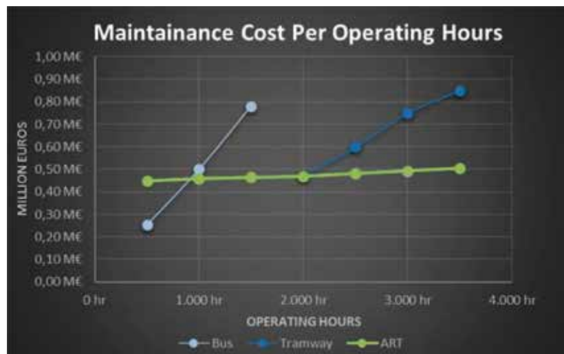
Figure 3: Comparison between operational costs of Buses, Trams and ART systems. Source: Author (Figure 6, El Jouzou, WTPP: 22.4).
