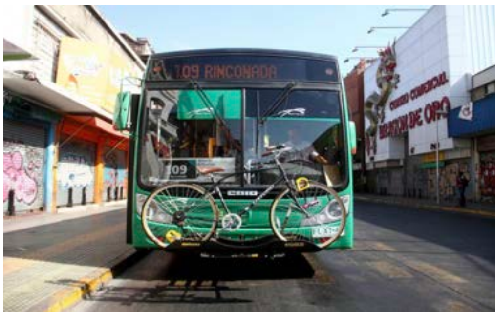
Figure 3. A BiciBus vehicle with a front-loading rack (Source: FMDOS)
