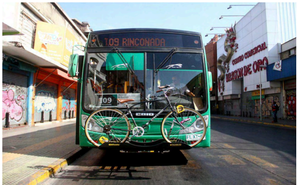
Figure 3. A BiciBus vehicle with a front-loading rack (Source: FMDOS)
